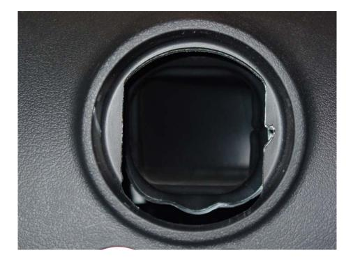
3. Place vent block (4 <sup>1</sup>/<sub>2</sub>" square foam) into plastic vent opening. Do not push foam in to far, as it will block next vent over. Just try to seal off the vent. You check for position by turning on the AC fan. A very small amount of air may still be detectable.
